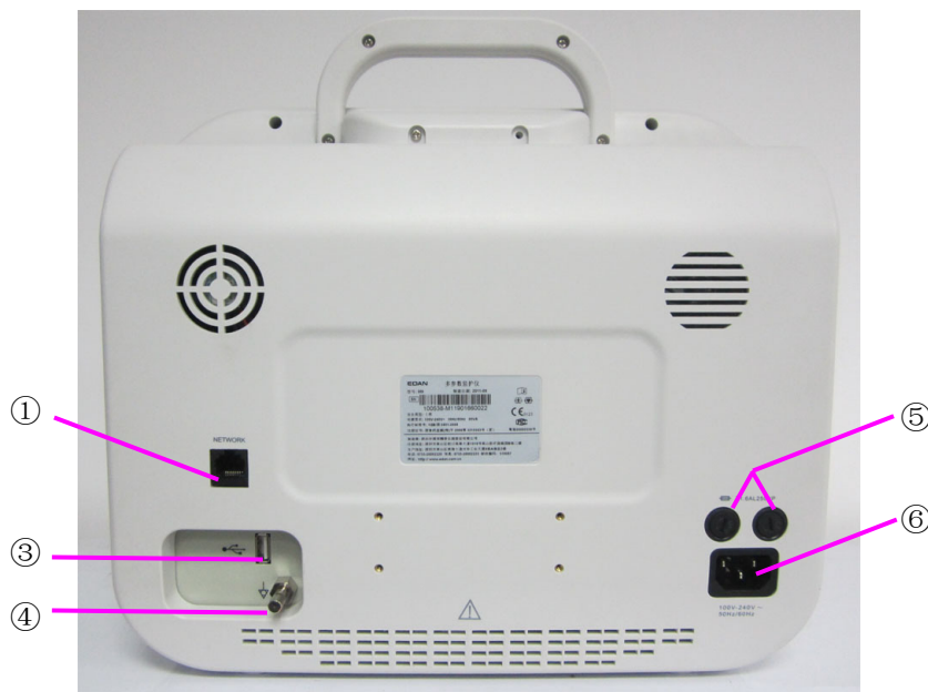
Figure 3-14 Rear Panel of iM9 and iM9A
