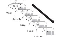
**3.** Press the [START/STOP] button to store the setting. It automatically turns off after 3 seconds
