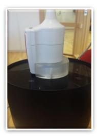
Insert the probe into the lid, ensure the probe leans against the probe holder.
