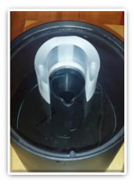
Place the lid firmly on the tank, with the probe holder up.
