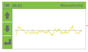
A flattened PVR waveform or a PVR without the typical shape is an indicator of severe PAD. The absence of the pulsations caused by occlusions in the artery makes it impossible to calculate the ankle pressures. Instead of ABI value, the device will display a "PAD" result, indicating severe disease. The result is confirmed with non-typical, flattened PVR waveform, similar to the picture on the left.
